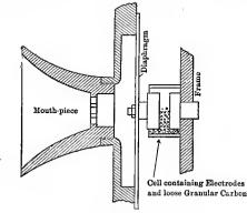
FIG. 176. Essential parts of Granular Carbon Telephone Transmitter.
